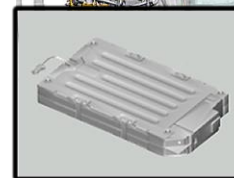
(a) 12V Auxiliary Battery (Main)
